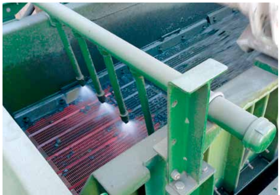
Linear motion conveys trash and debris off screen surface and into collection bins
