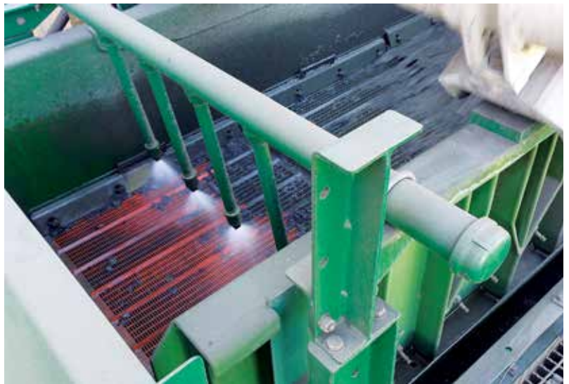
Optional wash system for further rinsing of concentrate from trash
