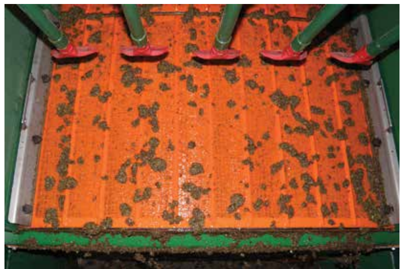
Derrick Polyweb® urethane screens recovering plant matter from process water at 500 microns
