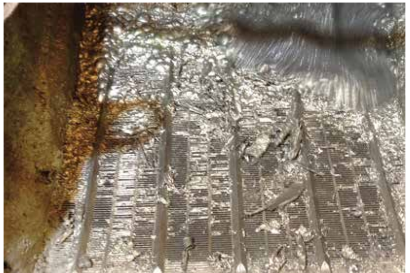
Copper concentrate screened at 1mm prior to column cell flotation
