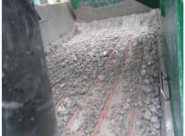
Derrick FLC 2000 shaker in operation
