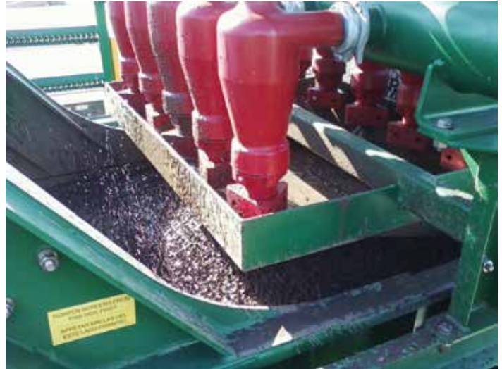
Derrick hydrocyclones operating on the FLC 423
