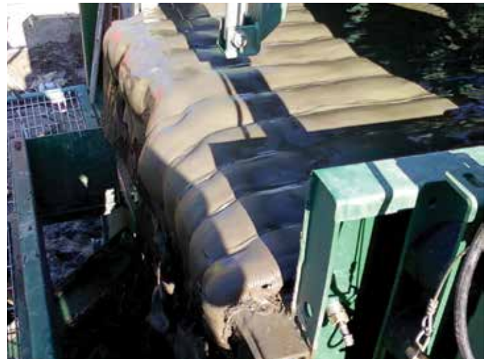
Dewatered solids off the FLC 423 deck
