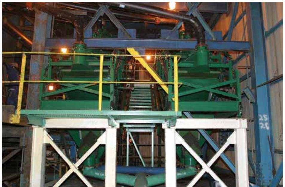
Figure 1. Leatherwood Stack Sizer installation
